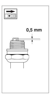
If the machine is low on power, difficult to start or runs poorly while idling always check the spark plug first.
